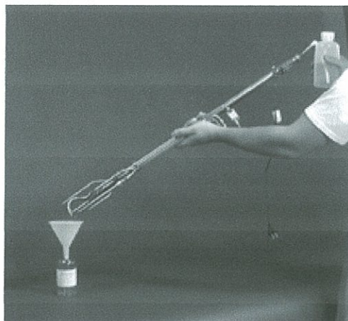
Figure 8-6. Acetone Rinse of Sampling Probe Liner
