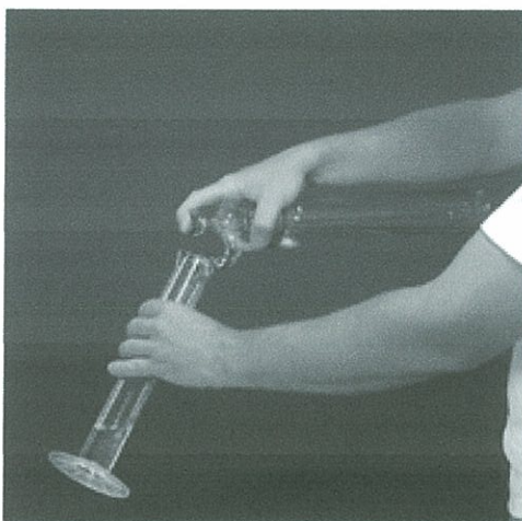
Figure 8-11. Measuring the Impinger Water Using Graduated Cylinder
